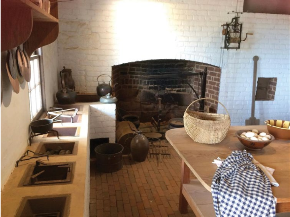
Figure 7.1 The kitchen at Monticello, Charlottesville, Virginia, USA, showing clockwise from left: a bank of stewing stoves, set kettle, fireplace with crane, roasting jack on the wall above, and beehive baking oven (closed). Photo: Jacqueline Newling 2018.
